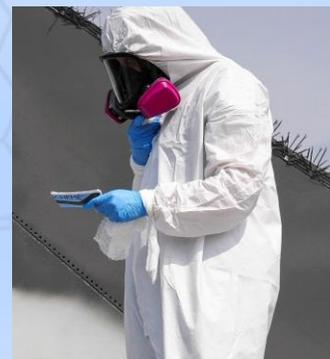
**Synthetic Blood Penetration Test ASTM F1862** was used to qualify our Biosafety hoods as level 1 and 2 barriers against blood splashes (at a distance of one foot and velocities corresponding to a human blood pressure of 80 and 120 mm Hg). **Please note:** nonwoven fiber-web structures are not water-proof and can be wetted through by detergents, pressurized liquids, high viscosity solutions and alcohol or other organic solvents.
